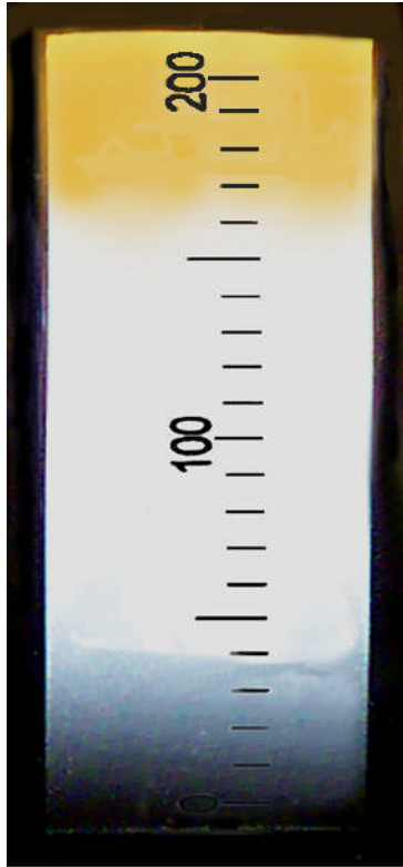
Cal-Gage before Analyzer Rotation (Black fringe is at zero nanometers on scale)
