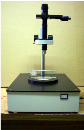
Figure 1. PS-100-MW polarimeter showing MWA-100 compensator and glass slice in proper position for measurement.
